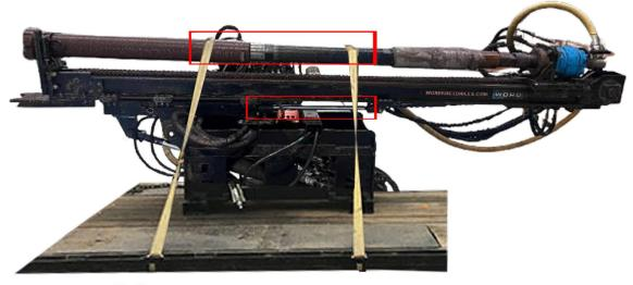
**X** DO NOT LEAVE FEED EXTEND CYLINDER EXTENDED WHEN SHIPPING TOOLING DO NOT STRAP OVER THE TOOLING
